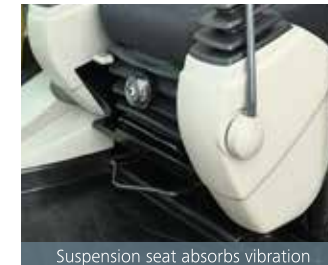
Suspension seat absorbs vibration
