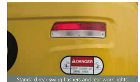
Standard rear swing flashers and rear work lights.
