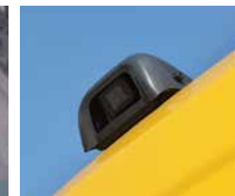
Standard rear-view camera eases safety checks behind the machine. Color video displays on cab monitor.
