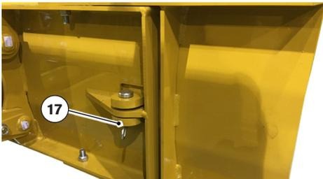
To swing the blade wings inward, pull the clevis pins (17) located on the back side of the blade. Simply turn the wings inward, reinstall the clevis pins at holes (18) located on top
