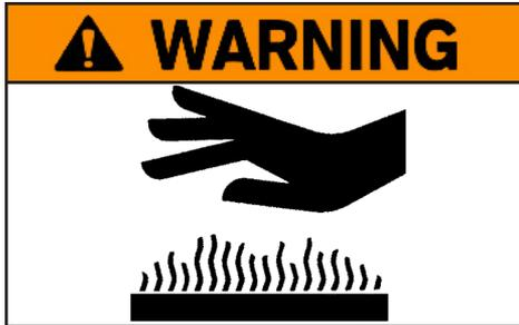
Do not touch any part of an operating engine. Allow the engine, radiator, exhaust and hydraulic reservoir to cool before any maintenance is performed. Relieve all pressure in the air system, oil system, lubrication system, fuel system, and/or in the cooling system before any lines, fittings or related items are disconnected.
