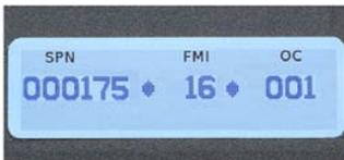
**Active Shutdown or Warning** screens display when a fault occurs. The screen lists the SPN, FMI, and Occurrence Count. If there is more than one fault, PV25 automatically scrolls through all faults.
