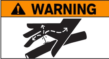
**Pressurized air and/or water can cause debris and/or hot water to be blown out.** This could result in personal injury. When pressurized air and/or pressurized water is used for cleaning, wear protective clothing, protective shoes, and eye protection. Eye protection includes goggles or a protective face shield.
