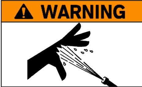
Check lines, tubes and hoses carefully. Do not use your bare hand to check for leaks. Use a board or cardboard to check for leaks. Tighten all connections to the recommended torque. Replace the parts if any of the following conditions are present:
